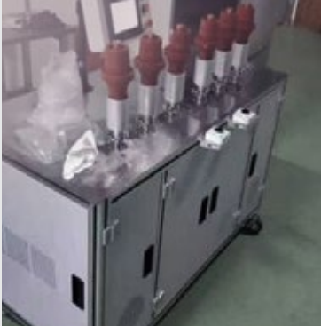
Electrical Insulation Components Detection
