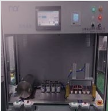
High voltage DC relay detection
